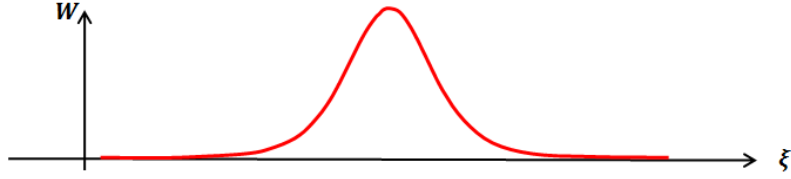
Figure 20: Soliton for the KdV equation.
