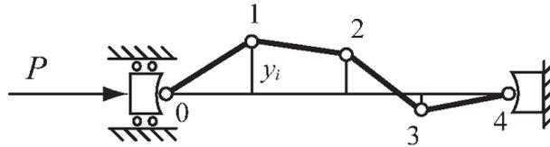
Figure 3. Simple model of a column loaded by an axial force.
