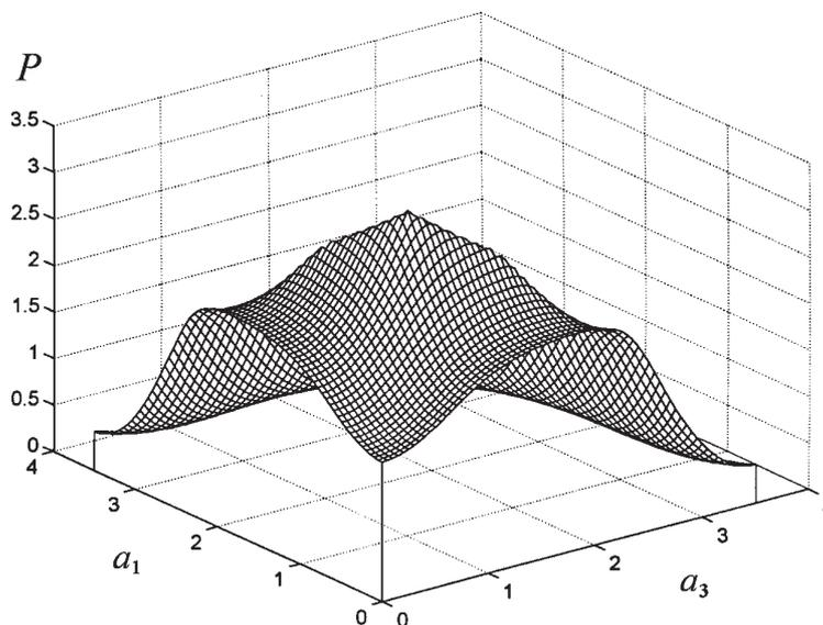
Figure 4. Stability boundary for the column in the parameter space  $\mathbf{p}$ .
