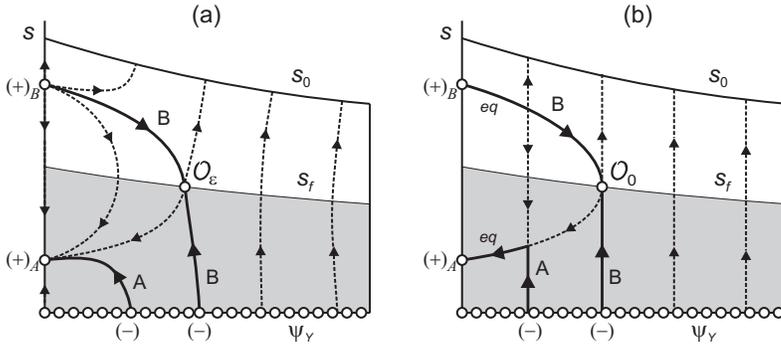
FIG. 4.2. (a) Orbit structure of system (4.23), (4.24) for  $v > v_0$  and small  $\varepsilon > 0$ . There is a single orbit  $B$  corresponding to a (resonant) traveling wave with the  $(+)_B$  limiting state, and a family of orbits  $A$  corresponding to traveling waves with the  $(+)_A$  limiting states. The arrows' directions correspond to increasing  $\tau$ . For increasing  $\xi$ , the arrows must be reversed in the upper (white) domain. (b) Singular limit  $\varepsilon \rightarrow 0$ .
