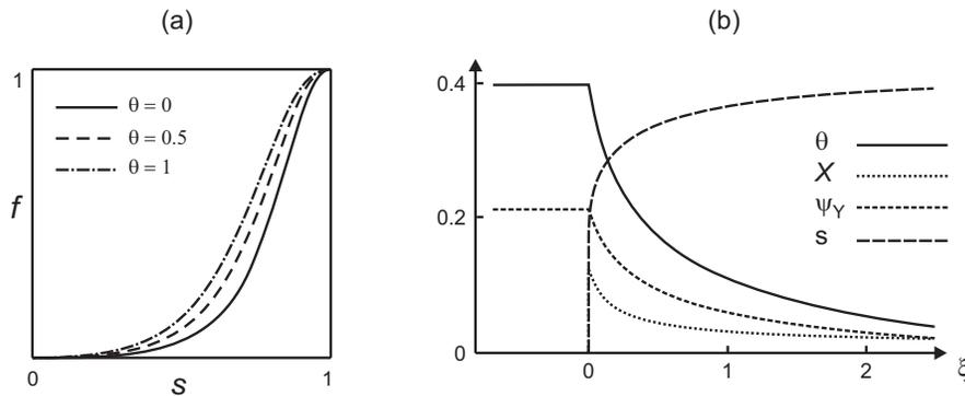
FIG. 6.1. (a) Fractional flow function  $f(s, \theta)$  for different  $\theta$ . (b) Resonant LTO wave profile in the limit  $\varepsilon \rightarrow 0$  for  $Y_{inj} = 0.21$  and reaction rate (6.2). The vaporization region reduces to a discontinuity of  $s$  and  $X$  at  $\xi = 0$ . The reaction region corresponds to  $\xi > 0$ .
