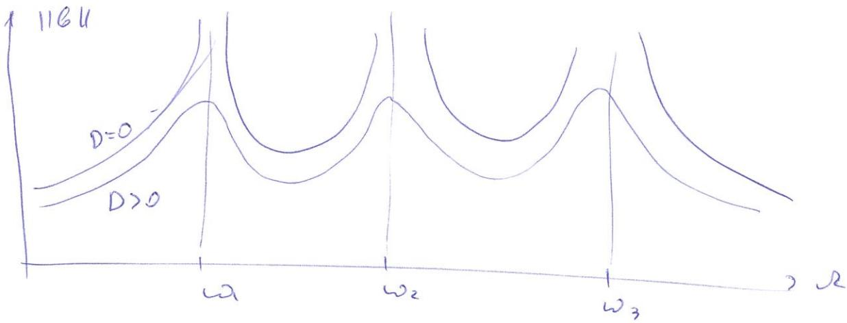
System with dissipation:  $M\ddot{x} + D\dot{x} + Cx = f_0 \cos \omega t$
