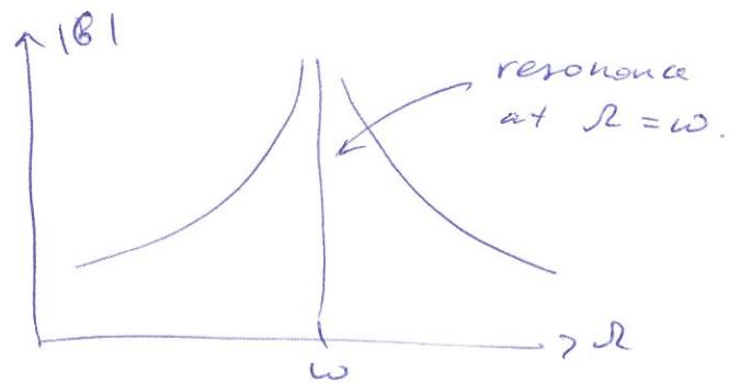
Oscillations near the resonance from the rest:
