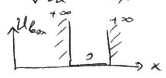
$$U_{\text{tot}} = \sum_{a=1}^N U_{\text{box}}(r_a), \quad U_{\text{box}}(r) = \begin{cases} 0, & r \text{ is in the box} \\ +\infty, & r \text{ is outside the box} \end{cases}$$
